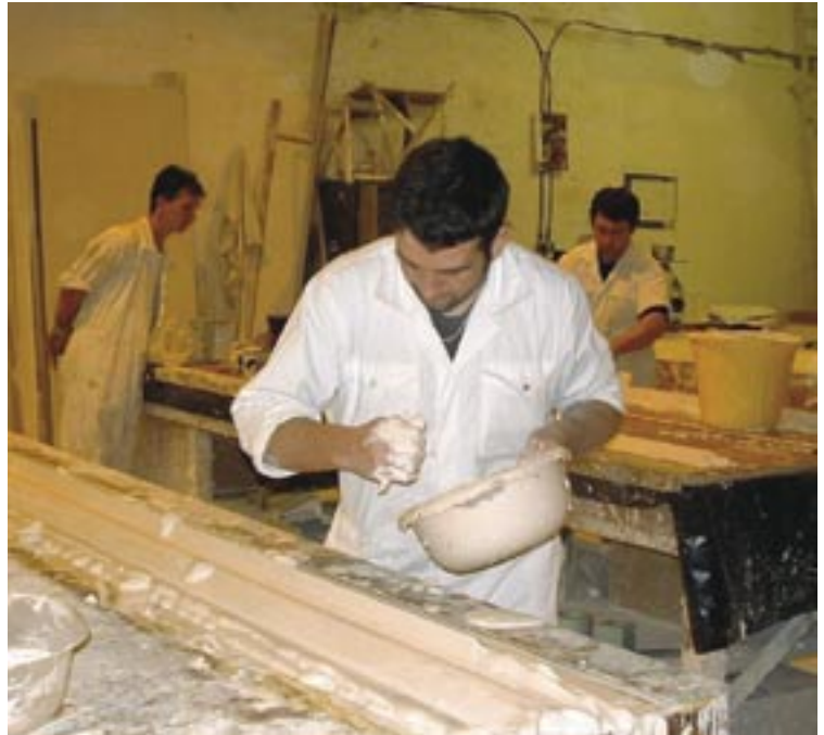
Phil Burkin running a mould at Troika Architectural Mouldings workshop in Sheffield.
